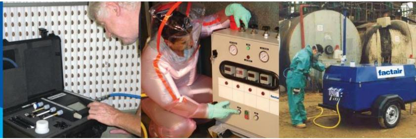
The Factair BAHP300EX is an electrically powered, HP breathing-air charging compressor designed to operate in a ATEX zone 1 hazardous area (ATEX marking:  $\text{Ex}$  II 2 G, Ex d IIB T3).
