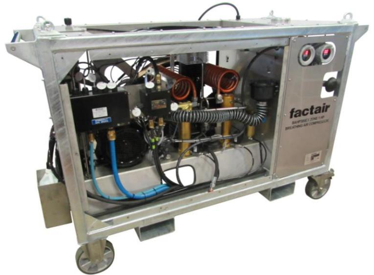
mains isolator, star/delta motor starter, automatic condensate drainage system, automatic stop on final pressure, display providing hours run and fault information and start/stop buttons.
