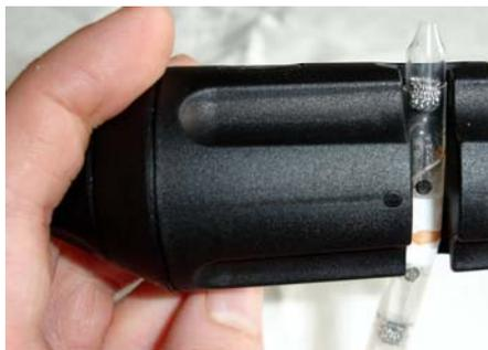
6. Place your used detector tubes in the F2154 Travel Container, until they can be disposed off properly as "sharps" or glass.
