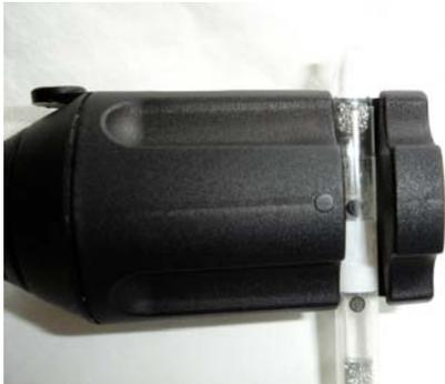
5. With one hand holding the cutter and the other holding the tube, applying pressure. This should break the inner tube.
