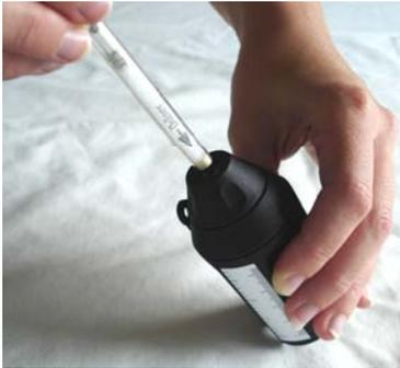
2. Push the tube at an angle to break the tip.
