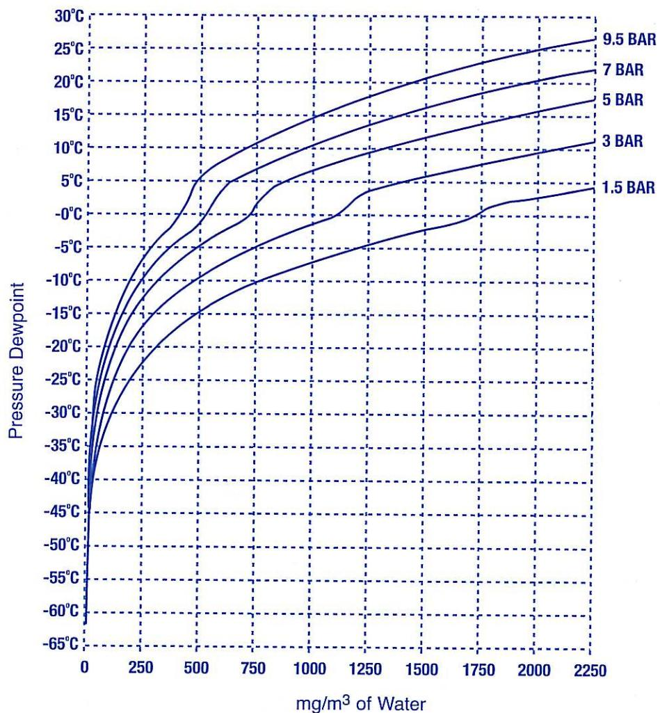
To establish pressure dewpoint take the point where tube reading in mg / m<sup>3</sup> intersects system pressure and read off pressure dewpoint from vertical scale.
