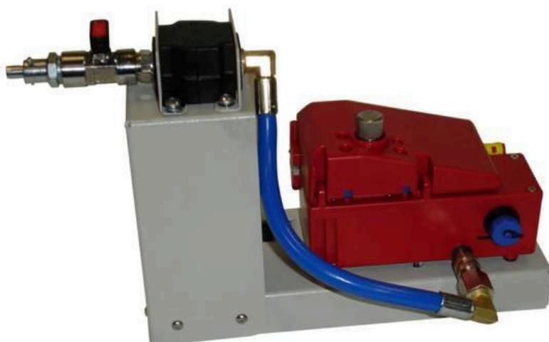
4A Blowing Head mounted on dispenser.
